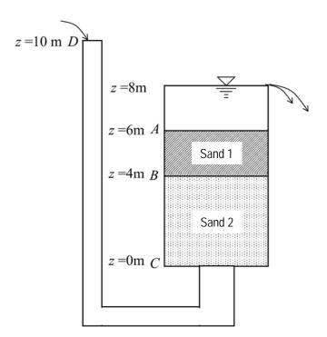
(4) Assume a new, homogeneous specimen, in which sand 1, in the figure, is replaced by sand 2. How further will point D need to rise to cause seepage failure (quicksand) of the sample?
